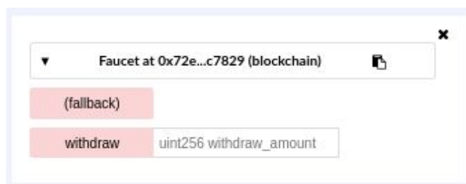
Figure 2-20. The withdraw function of Faucet.sol, in Remix
